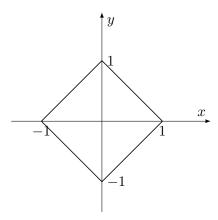
This shape is a square. We can think of it as made up of 4 right angled triangles, each with base and height equal to 1, so each has area  $\frac{1}{2} \times 1 \times 1 = \frac{1}{2}$ , and hence the square has area 2. Thus the correct option is C.
