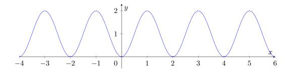
Finally, the graph of  $y = 2(1 - \cos(\pi x))$  is the previous graph scaled by a factor of 2 in the *y*-direction:
