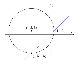
The region x > y is below this line, and we see that only part of the circle is included in the region. Since the points of intersection of the line x = y with the circle are at (1, 1) and (-5, -5), it is clear that exactly one quarter of the circle lies in the region x > y. Therefore the length of the curve with the given equation is  $\frac{1}{4}$  of the circumference of the circle, that is,  $\frac{1}{4} \times 12\pi = 3\pi$ , and the correct option is D.
